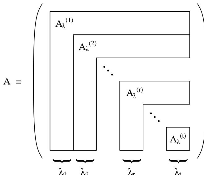
FIGURE 4. Adjacency matrix with block structure as used in Algorithm 2.9
