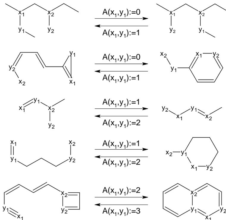
FIGURE 5. Examples of random displacements as used in Monte Carlo and simulated annealing algorithms
